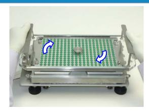
**11**. Hold Locking Plate by handles and twist clockwise to lock into place.
