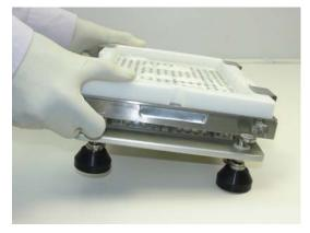
**18a.** Instead of tamping, hold Filler and gently tap against table a few times to settle powder. Powder Tray Clamps are recommended when tapping. Squeeze Cam Handle gently to hold bodies in Filler.
