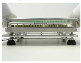
**13**. Push down on Locking Plate handles while pulling up on Locking Plate to separate capsule caps and bodies. Set aside Caps Tray with Locking Plate. See Tips #1 and 2.
