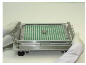
21. Repeat step 20 with hands positioned in opposite corners as shown. Repeat for the other 2 corners. Caps and bodies are now re-assembled. They are not fully locked. See Tip below.
