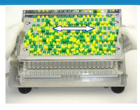
2. Fill Capsule Measuring Bowl for your capsule size and pour capsules on Orienter Tray. Lift Orienter Tray and shake back and forth moving capsules into slots.
