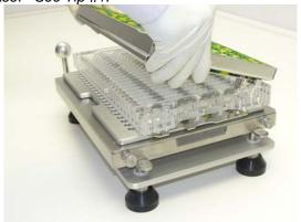
4. Place Orienter Tray onto Orienter Base by sliding into 2 grooves on sides of Orienter Base.
