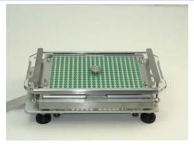
**19.** Remove Powder Tray. Place Caps Tray with Locking Plate onto Filler.
