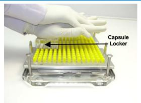
**22.** Remove Caps Tray with Locking Plate and turn them over onto table. Use 25-hole Capsule Locker to lock capsules. Apply pressure with both hands until you feel the capsules snap and lock. Holes in Caps Tray help guide Capsule Locker position.
