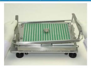
**10**. Hold Locking Plate by its 2 handles and place onto Caps Tray. The 4 posts of the Caps Tray should enter 4 larger holes in Locking Plate.
