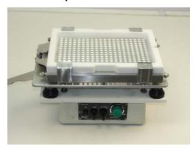
**18c.** Use optional Vibrator as an alternative to tamping or tapping (see pages 16 & 32). Powder Tray Clamps are recommended.
