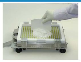
**17.** Pour pre-measured powder onto Filler. (For overfilling capsules, *see Tip #1*). Use Powder Spreader to move powder from center towards all 4 edges of Powder Tray frame.
