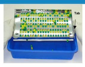
3. Tilt Orienter Tray and press tab down to lift gate and pour off excess capsules. See Tip #2.
