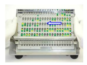
5. Push sliding portion of Orienter Tray to the left to 6. Move Orienter Base with Orienter Tray to drop capsules into Caps Tray, filling every third row. Position II on Caps Tray. See Tips #3, 4, 5.
